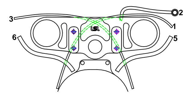
Throttle cable (1): Route the throttle cable in front of the right stanchion and afterwards under the spacer of ignition lock, between ignition lock and steering head tube, back to the instruments. Fix the cable with cable strap on the steering head tube (upper fixing point of the cockpit bracket). Make sure, that no cable is bended, also with full steering.
