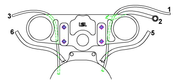
**Throttle cable (1):** There is no rerouting necessary. Check throttle cable for free movement on every steering angle.
