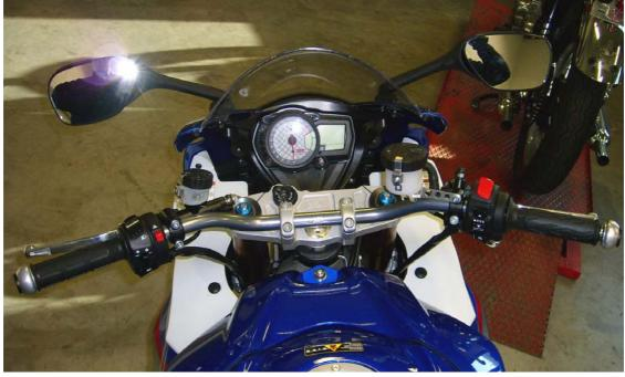
(D) Remove the fuel tank first to avoid scratches and dents when re-routing hoses and cables. Remove fairing bracket and mirrors if necessary. The battery ground should be disconnected before working on electric wiring and switches!
