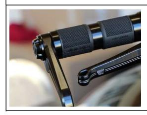
Caution: Make sure there is sufficient space between the mirror and the other parts (also with maximum steering angle).
