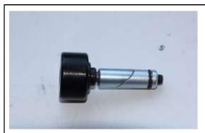
Remove the original handlebar weights and dismantle.
