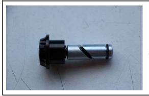
Mount and align the mirror with the bar end and the original screw to the handlebar.
