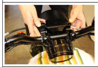
... and place the pre-assembled clamps onto the triple clamp.
