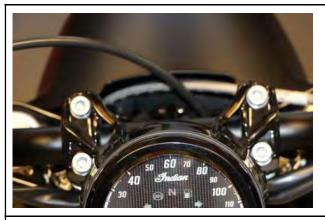
Loosen the four screws of the clamps. Unplug the speedometer or place on tank.
