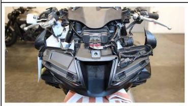
Remove the left and right side covers, the plastic covering under the head-lamps as well as the windscreen and front fairing according to manufacturer's specifications.
