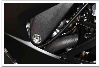
The clutch cable is laid under the motor mount.
