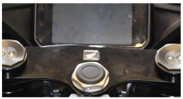
Attach top yoke with the original nut and the two screws for the fork (torque according to manufacturer's specifications).
