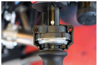
Before the final fixing of the handlebar and the switch units, make sure that there is no contact with any other parts when the handlebar is in its maximum steering angle.
