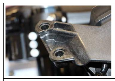
Remove all four spacer sleeves from the fairing holder.
