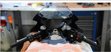
Cover all parts in the handlebar area (tank cover, speedometer, left and right side cover).
