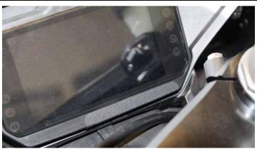
If necessary, cut the scoring protection for the display and stick it on its border.
