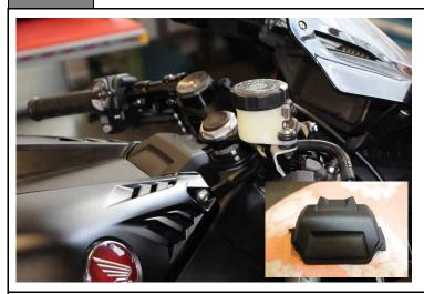
Remove the front tank fairing and the steering lock cover.
