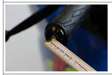
Evenly adjust the distances of the handlebar ends on both sides ...
