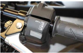
Align the throttle grip and switch units on the handlebar.
