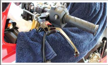
On the left, slide clutch lever and switch unit onto the handlebar and stick on the rubber grip.
