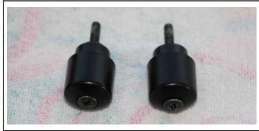
Remove both handlebar ends. Remove the left-hand rubber grip from the handlebar with compressed air.
