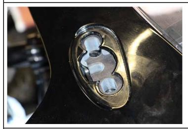
Carefully slide the fairing pad between the holder and the fairing.
