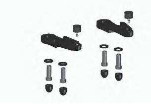
Screw the provided rubber buffer into the fairing pad from above.
