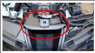
Remove the original rubber bearing at the fairing holder.
