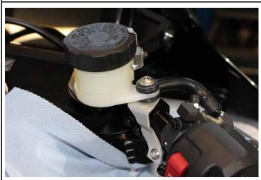
Mount the original container onto the lower fixing point of the brake pump using the enclosed screw and spacer sleeve.
