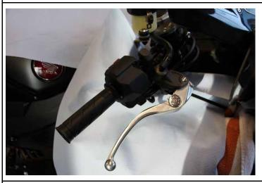
Mount the hand pump onto the handlebar.
