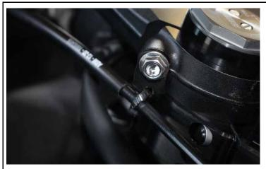
Increase the bigger hole ( $\emptyset$  6.5 mm) of the holder provided to  $\emptyset$  8.0 mm with a drill. Attach the holder to the left top yoke screw.
