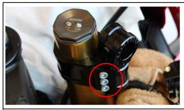
Slide the clamps of the multiClip onto the fork.
