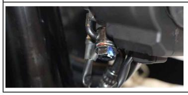
Tip: Lightly loosen the fixing screw of the brake line at the hand pump and reattach by hand.
