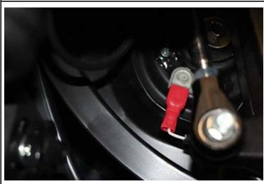
Connect the cable extension to the horn.
