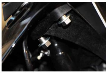
Insert the indicators on both sides as per original, place the mirrors from above and loosely screw in the provided nuts and washers (with thread-locking fluid) into the fairing holder from beneath.
