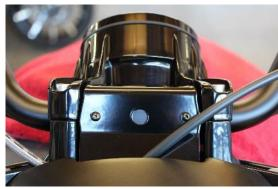
Attach the cover to the holder with the screws provided.
