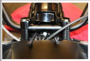
Lay both cable ties around the handlebars as shown in the image.
