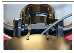
Fasten the holder to the handlebar using cable ties.
