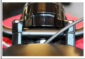
Clean the surface of the handlebars between the clamps.
