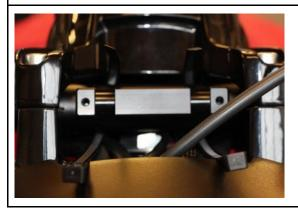
Place the holder in the middle of the handlebar. Align the threaded holes to the front.
