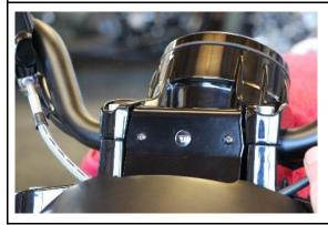
Stick the pin into the notch and remove the protective film.
