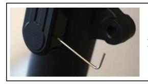
Attach the cover with the thread pins provided, using thread-locking fluid (medium strength).
