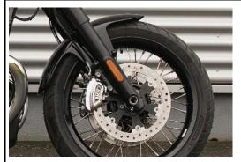
Cover the fork in the area around the side reflector to protect against damage.
