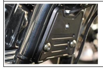
Mount the cover with the enclosed screws.
