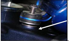
Install the K-washers under the tank mount with the provided bolts.
