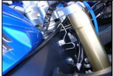
Relocate inside and use the holder that was previously used for the throttle cable. This holder will need to be twisted slightly.
