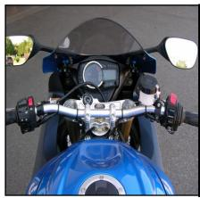
For the final assembly of the controls it is necessary to drill holes for the centering pins. To do this, align the controls and mark the position of the centering pins (use a center punch to mark the location) and then drill a hole. Make certian the hole diameter and depth correspond to the centering pin.
