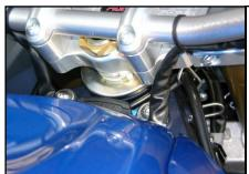
Route the wiring for the right and left controls under the tank and in front of the airbox.
