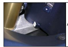
Attach the steering stop to the stop with the supplied adhesive.
