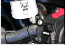
Secure the brake reservoir with the provided bracket and bolt.
