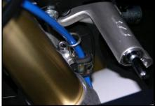
Route the new steel braided brake lines according to the assembly instructions.
