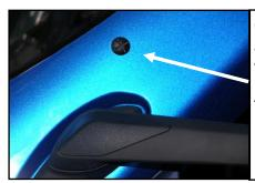
Guide the turn signal wire through the middle hole of the underlay and then route it inwards through the cut out between the rubber and the underlay so that it is not pinched.
