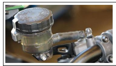
After installation of the brake line and master cylinder the brake fluid reservoir bracket has to be aligned in order to be level.
