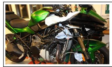
Remove right fairing and the cover underneath the headlight.
