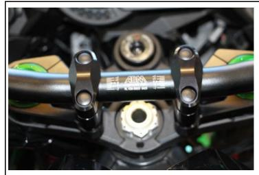
Align the handlebar with the adapter clamps and tighten slightly up the riser clamps.
