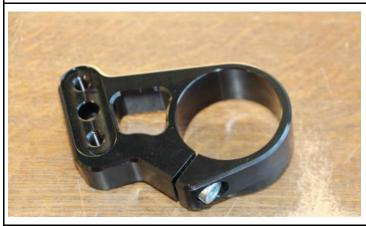
Install the riser clamps utilizing the supplied the M10 bolts and Schnorr-safety washer (use also thread locker) at the triple clamp with 28Nm.
