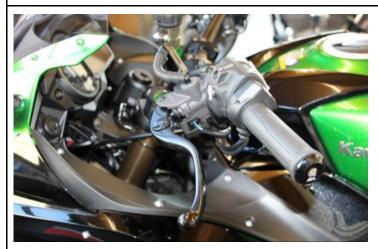
The brake line routes from the ABS unit straight to the master cylinder.
