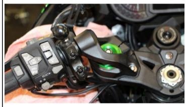
Remove all controls and the throttle cables from the original handlebars.
