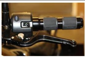
Slide the clutch handle onto the handlebar and fasten from below using the three thread pins.
