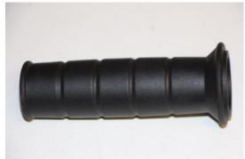
Loosen the rubber grip on the left side using compressed air and remove.
