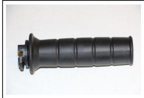
Push the armature slightly forwards, unclip the original grip and remove completely.
