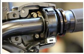
Apply some grease onto the handlebar in the throttle area.
