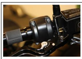
Remove the four screws of the right armature and unclip the front switch unit.
