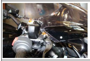
Align the brake, clutch and handlebar switch and turn the handlebar left and right.
