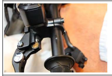
Now, centre-punch the marked position and drill a hole (diameter and depth are based on the centring pin).
