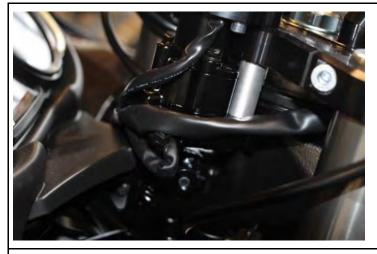
The cable of the clutch handlebar switch is laid to the right under the top yoke but above the speedometer bracket.
