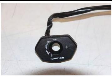
Loosen the screws of the immobiliser and remove them from the top yoke.
