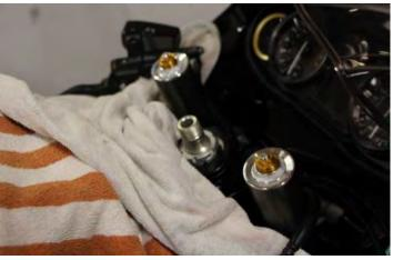
Pull the top yoke off the fork. Pull the accelerator grip off the clip on.
