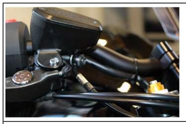
Attach the brake line with the new seals onto the hand pump.
