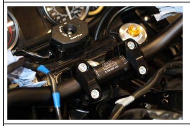
Slide the accelerator grip onto the handlebar, adjust the handlebar (see image) and lightly fasten it with the clamps.
