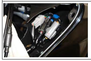
Unplug the plugs for the handlebar switches and the ignition lock under the right cover.
