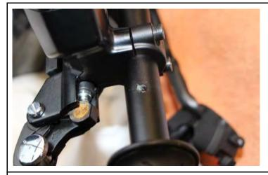
The final assembly of the handlebar switches requires the drilling of holes for the centring pins.
