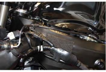
Completely remove the two original brackets and the clutch line.
