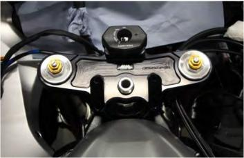
Attached the top yoke with the original nut and washer.
