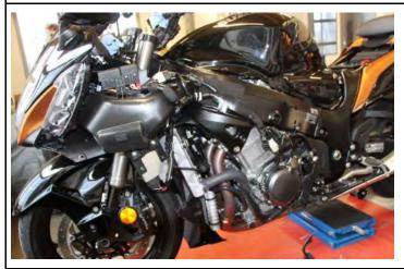
Remove the entire left side fairing according to manufacturer's specifications.
