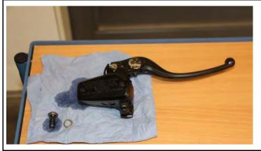
Drain the brake fluid according to the manufacturer's specifications.
