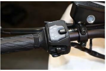
Stick on the left rubber grip flush to the handlebar.
