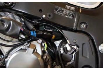
Attach the clutch line with new seals to the hand pump and cylinder.
