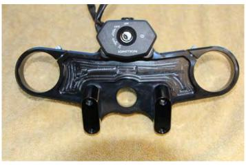
Screw the inclined clamps with the screws (M10), Schnorr safety washers and thread-locking fluid onto the top yoke.
