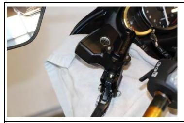
Drain the clutch fluid according to the manufacturer's specifications.
