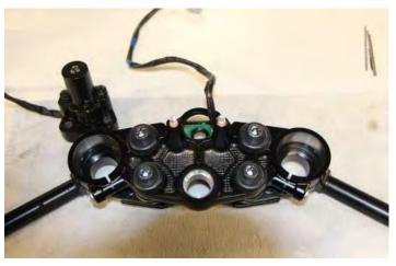
Loosen the screws of the ignition lock using a special tool or drill out.
