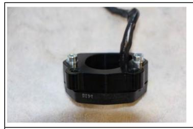
Attach the immobiliser to the bracket using the screws and washers provided.
