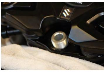
Remove the nut of the top yoke and loosen the clamp screws.
