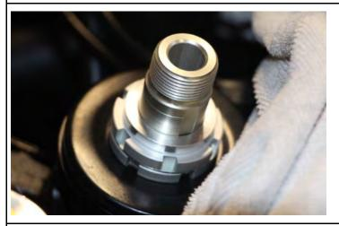
Place the spacer ring provided onto the head tube.
