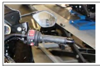
Mount the handlebar end onto the accelerator grip side.
