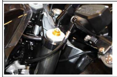
After mounting the clutch line, the complete unit must be drainer according to manufacturer's specifications.
