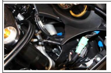
Loosen the two cable harness brackets on the right under the fairing.
