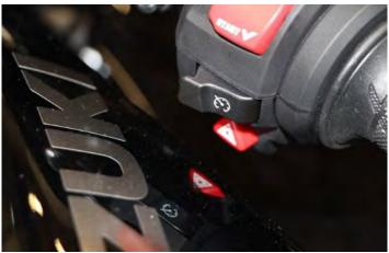
In doing so, the handlebar and the handlebar switches must not touch other components (e.g. fairing or tank), even with the handlebar turned fully.
