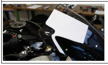
Place the template onto the fairing and draw on.
