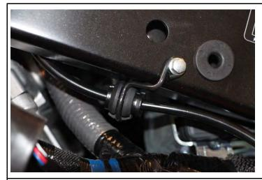
Slide the rubber mounts onto the new clutch line and attach using the original brackets.
