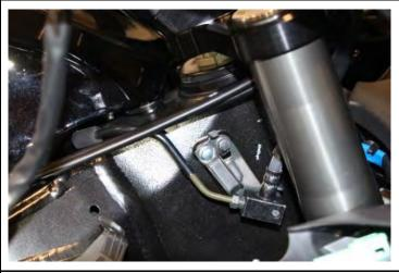
Lay the accelerator cables over the steel line.
