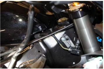
Remove the retaining plate for the accelerator cables.
