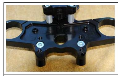
Tightening torque 28 Nm
