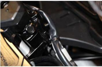
Attach the cable of the ignition lock, immobiliser and clutch handlebar switch to the ignition lock with a cable tie.
