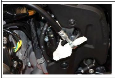
Loosen the connection of the clutch line from the slave cylinder.
