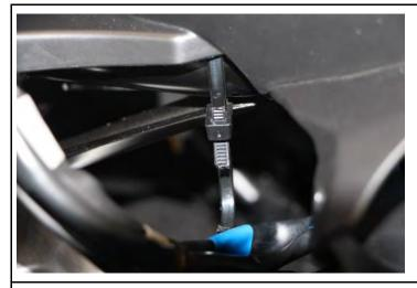
Unclip the cable harnesses on the right side from the two brackets.
