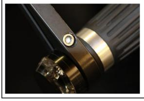
Tighten the clamp screw on the supporting arm.
