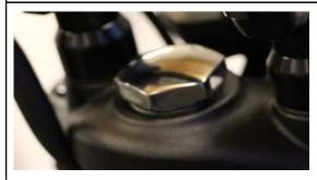
Loosen the nut of the triple clamp.
