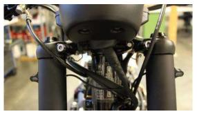
Carefully slide the triple clamp onto the fork.
