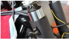
Slide an O-ring onto both fork tubes down to the cover.
