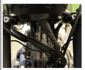
Cover both indicator cables with the long heat-shrink tubing and shrink using a heatgun.
