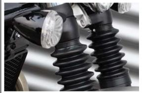
Loosen the clamp screws of the indicators and disconnect their cables (left).
