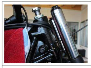
Carefully pull the triple clamp off the yoke and place onto the towel.
