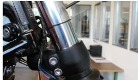
Slide an O-ring (2mm diameter) onto each fork tube down to the lower triple clamp.
