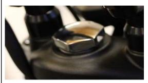
Attach the yoke nut. Torque 65 Nm
