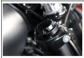
Clamp the covers with the thread pins provided to the fork
