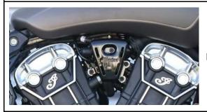
Loosen the four fixing screws of the original cover.
