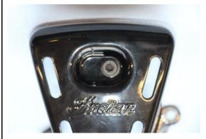
Insert the screw in the centre of the original cover.
