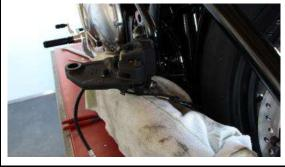
Pull the brake caliper out to the front and carefully place it down.
