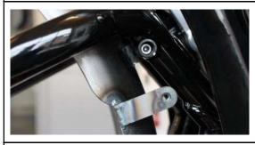
Carefully slide the fender into the swingarm and fasten with the original screws.
