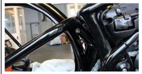
Loosen the six fixing screws of the fender and ...
