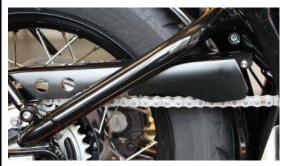
Completely remove the chain guard.
