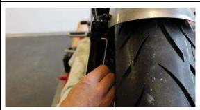
The thread pin on the arm enables further slight adjusting of the fender and the rear lights.
