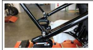
Attach the two braces with the chain guard to the swingarm. Attach the chain guard to the in the front at the fender.
