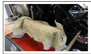
Cover the exhaust and frame on both sides with a cloth.
