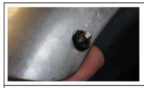
Attach the braces with the screws, washers and o-rings...
