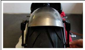
Align the fender and fasten all screws. Align the previously mounted spacer sleeves to the fender.
