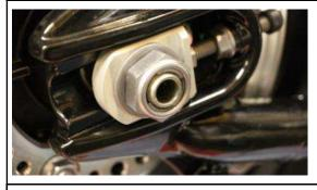
Dismantle the right-hand axle nut with washer and chain adjuster and remove the axle (including the left-hand chain adjuster).
