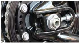
Push in the axle (including left-hand chain adjuster) through the swingarm and the rear wheel.
