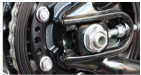
Push in the axle (including left-hand chain adjuster) through the swingarm and the rear wheel.
