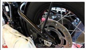
Run both cable harnesses under the swingarm and connect them to the original plugs above the battery. The setting for the blinking frequency of the LED indicators has to be done by a Triumph dealer. Attach the cables with the cable ties.
