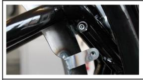
Carefully slide the fender into the swingarm and fasten with the original screws.
