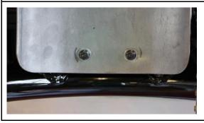
Lightly attach the hexagon screws (M6) with the spacer sleeves and the original washers.
