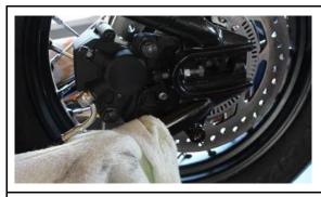
Remount the rear wheel and mount the brake caliper according to the workshop specifications to the swingarm.
