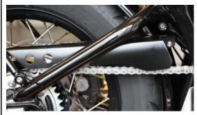
Completely remove the chain guard.
