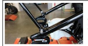
Attach the two braces with the chain guard to the swingarm. Attach the chain guard to the in the front at the fender.
