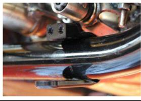
Insert the adhesive rubber into the rounding of the front holder and slide onto the frame at the mounting position at the baseplate.
