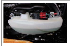
Reattach the coolant reservoir, making sure that the ring cable lug of the provided ground cable is attached on the right side under the lock nut.
