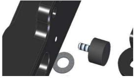
Screw the rubber buffer (provided) into the baseplate using thread-locking fluid and hand tighten.
