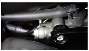
Drain brake fluid at the rear brake cylinder according to the workshop manual.
