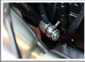
Insert the new brake light switch (provided) with a seal through the fitting of the original brake line.
