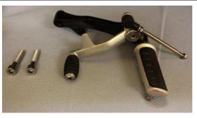
Remove the complete footrest system on the left-hand side as shown in the illustration.
