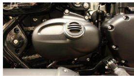
Completely remove the sprocket cover.
