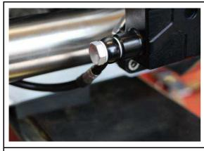
...it can be screwed onto the brake cylinder using the banjo bolt and seals provided.
