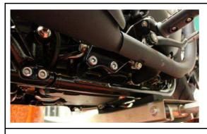
Loosen both fixing screws of the original footrest and remove it completely.
