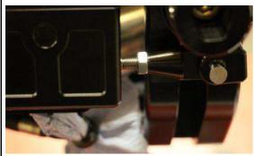
By changing the position of the push rod, the height of the foot brake lever can be finely adjusted.
