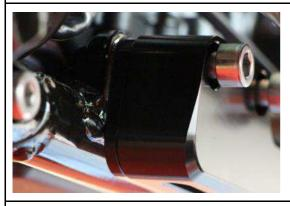
Lightly mount the baseplate with the two original screws...
