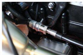
Screw on the new brake line with a seal onto the brake light switch.
