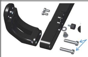
Attach the support bracket with the two screws (provided) to the baseplate.
