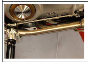
Screw on the shift linkage on both hinges, adjust the height of the gear lever and lock with nuts.
