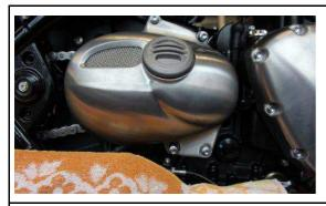
Reassemble the cover and all removed parts on the right side.
