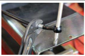
Turn the fitting of the brake line so that...
