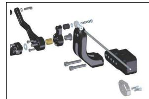
Attach the support bracket onto the baseplate, as on the right side.
