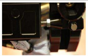
Screw the push rod into the link of the brake lever.
