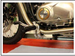
Attach the new system to the frame using the original screws.
