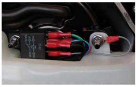
Mount the relay onto the holder where the original brake fluid reservoir was attached.
