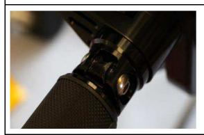
Attach the footrest with the threaded bush, the plastic washers and two screws (use thread locking fluid).
