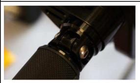
Screw the pedal onto the brake lever. Torque 10 Nm
