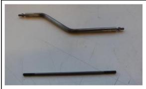
Unscrew the two nuts from the original shift linkage and screw them onto the one provided.
