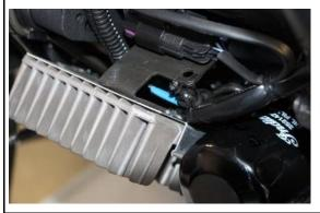
Remove the cable tie holder from the rectifier holder.
