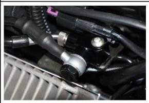
... and mount the manifold with the screw and nut provided.
