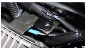
Place the spacer plate provided onto the holder...
