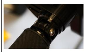
Attach the footrest joint with the threaded bush, the plastic washers (moisten with grease) and both screws (M8).
