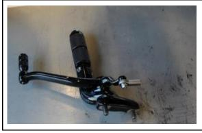
Remove the ball joint from the gear lever.
