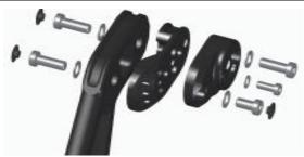
Attach the footrest mounting onto the adjusting plate using the screws and safety washers provided.
