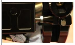
Screw the push rod into the tappet, align and fasten using the nut.
