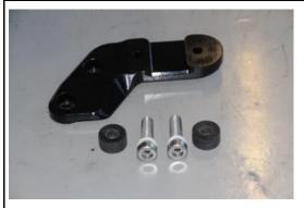
Attach the right baseplate to the frame using the two screws, safety washers and spacer bushings provided. Tightening torque 30 Nm
