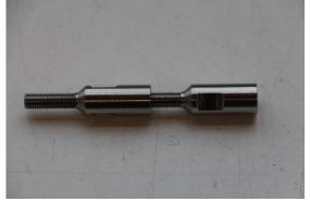
Caution: When mounted into mid or front position, one or two extensions must be used to mount the gear change rod.
