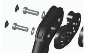
Attach the adjusting plate onto the baseplate with the screws and safety washers provided.
