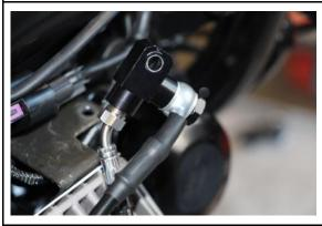
Attach the original brake line with new seals onto the manifold.
