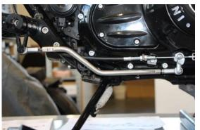
Screw the two original ball joint heads onto the shift linkage.
