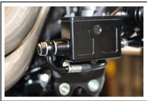
Screw the 90° connection onto the foot brake cylinder using two new seals.
