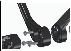
Bigger changes to the brake lever can be achieved by removing the lever and twisting it to the reversing lever. During the subsequent installation, note the following tightening torques:
