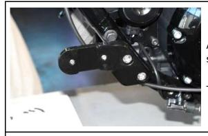
Attach the left baseplate to the frame using the two screws, safety washers and spacer bushings provided.
