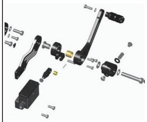
Firmly screw the brake lever to the reversing lever.
