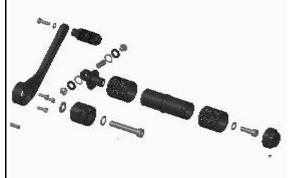
Adjust footrests with the inside screw (M8). Tightening torque 12 Nm
