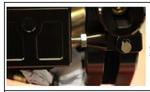
By screwing in and unscrewing the push rod, the position of the brake lever can be adjusted exactly. Then counter the push rod with the nut.
