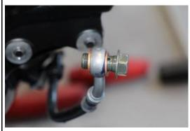
Drain brake fluid at the rear brake according to the workshop manual.
