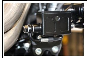
Attach the foot brake cylinder onto the bracket.
