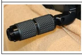
Reattach both covers using thread-locking fluid and the thread pin.
