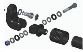
Insert each replacement footrest with four spring washers and two plastic washer into the mountings.
