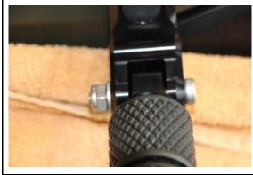
Push the screw and washer provided through the joint and attach using the nut in such a way that the joint can still be moved.
