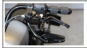
Attach the mirrors (using M10x1.25) to the clamps.
