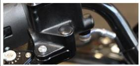
Remove the original mirrors and push the plastic coverings provided into the thread.
