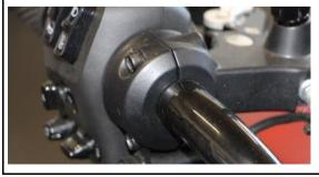
Remove the two original clamps and attach the mirror clamps using the original screws.
