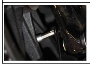
Attach the cover to the swingarm using the two original screws.
