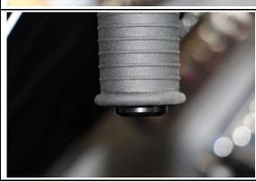
Push the switch units onto the handlebar until the handlebar extensions protrude approx. 2-4mm.
