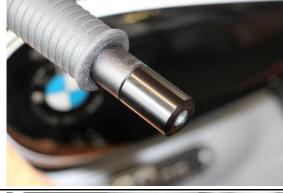
Attach the handlebar extensions provided on both sides and fasten.
