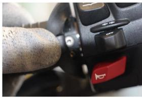
Dismantle the housing of the switch units on both sides, loosen the fixing screws and unplug the plugs of the units.
