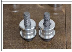
Remove the original screws and bushings.
