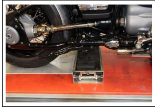
Make sure that the motorbike is securely positioned.
