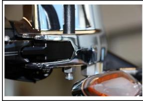
Attach the mirrors using the washers and nuts provided.
