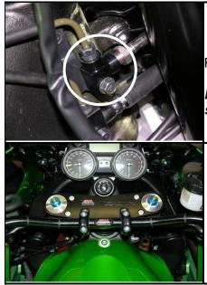
Remove the original brake line from the manifold.
