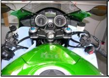
Loosen handlebar ends, grips, controls and handlebar stubs.
