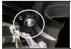
Attach the steering stops to the lower fairing bracket using the supplied bolts, washers, and nut.
