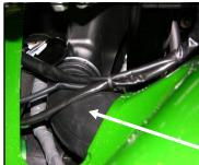
Unplug all connections underneath the black panel. Pull the cable out from under the air intake tube. (This will be routed over the intake tube during assembly.)
