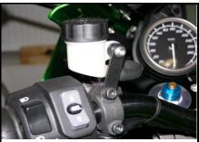
Fasten the clutch reservoir to the clamp using the supplied bracket, spacer, and nut. Verify that the reservoir hose is not kinked. The bracket may need to be bent a bit for installation.
