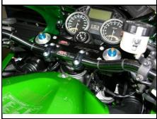
For the final assembly of the controls, it is necessary to drill holes for the centering pins. To do this, align the controls and mark the position of the centering pins (use a center punch to mark the location) and then drill a hole. Make sure that the hole diameter and depth correspond to the centering pin.
