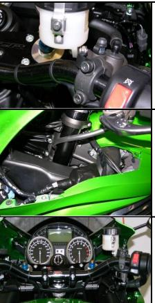
Fasten the brake reservoir to the lever clamp using the supplied bracket, bolt, washers, and nut. Make sure that the reservoir hose is not kinked. It may be necessary to bend the bracket a bit.
