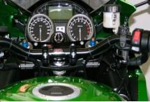
Install the throttle grip so that the cables are pointing down. Install the controls to the handlebars with the supplied cable ties and insert the cable via the air duct as shown.
