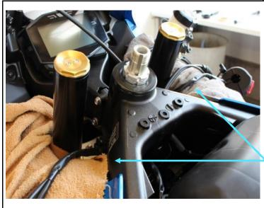
Remove steering stem nut and loosen up the upper pinch bolts for the fork legs
