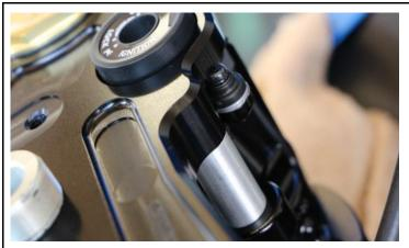
Remove the ignition lock from the upper triple clamp. Either drill out the bolt heads or remove them with a special tool.
