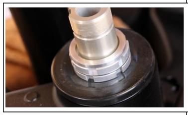
Slide the supplied aluminum spacer ring over the steering stem.
