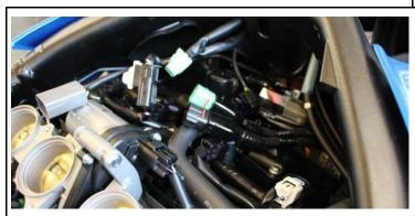
Remove the upper injection rail and the complete airbox.
