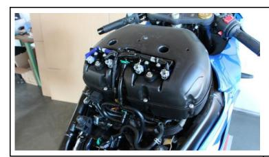
Remove seat, both tank covers and the tank
