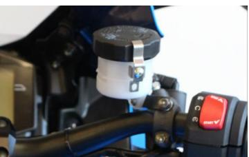
Mount the original brake fluid reservoir with the supplied bracket using the supplied longer bolt, washer and hex nut.
