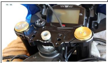
Install triple clamp with the original steering stem nut and spacer ring. Apply torque settings in reference to the manufacturers shop manual.
