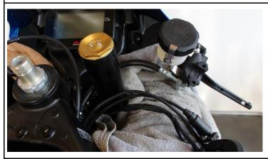
Drain brake fluid out of the master cylinder. Cover up the related work area.
