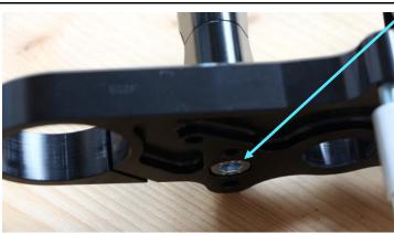
Install the riser clamps utilizing the supplied the M10 bolts and Schnorr-safety washer at the triple clamp with 28Nm. The wider side of the riser clamps point forwards!
