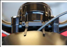
Fix the holder to the handlebars with the cable ties.
