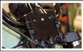
Attach the cover to the holder with the enclosed screws.
