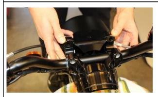
Insert the handlebars into the risers and align as desired.
