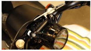
Lift the handlebars and place the risers on the triple clamp.
