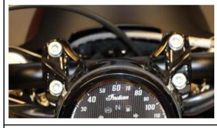
Loosen the four screws of the clamps. Unplug the speedometer or place it on the tank.
