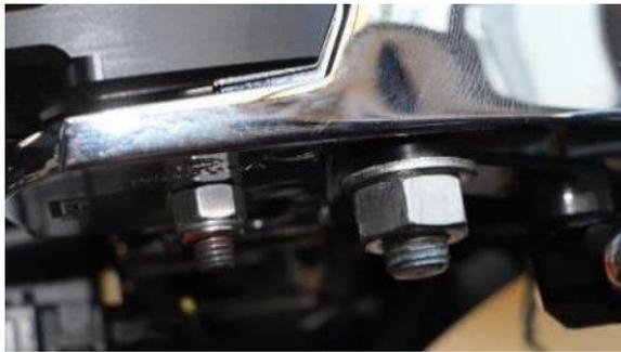
Adjust the mirror and indicator holder as desired and fasten the nut according to the manufacturer's specifications.
