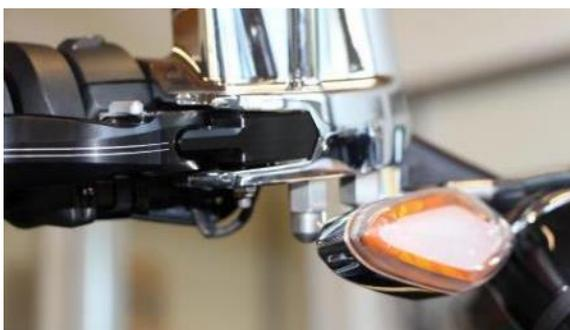
Loosen both nuts of the mirrors.
