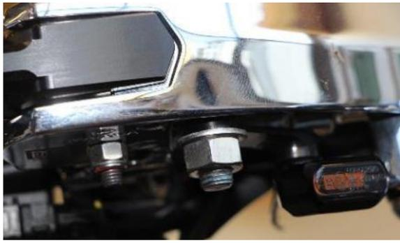
Push the indicator holder onto the mirror thread and lightly fasten using the original washer and nut.
