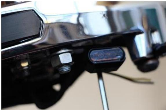
Align the indicator housing and fasten using the screw (M4). Solder both cable ends together. Use the heat-shrink tubing provided.
