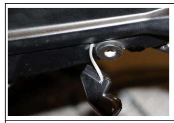
Guide the cables of the indicator over or through the rear the frame (drilling Ø 4 mm).
