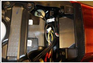
Connect the indicators and resistors supplied...
