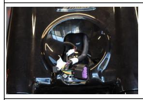
Unplug the headlight cable and remove the headlight.
