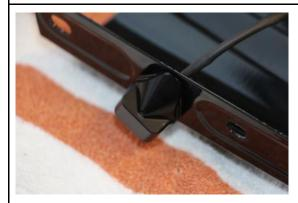
Guide the indicator cable through the sheet covering.
