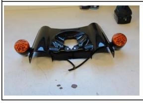
Remove the sheet covering and unscrew the original indicators.
