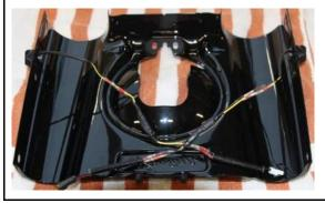
Push the sheet covering into the rubber guide of the top yoke.
