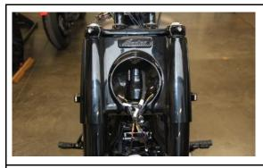
Attach the sheet covering to the headlight bracket.
