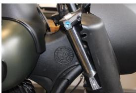
Disconnect the left and right indicators behind the headlight and remove completely including bracket.
