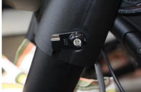
Mount the indicators with the brackets provided, align and attach all six screws of the headlight covering.
