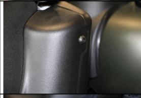
Carefully reattach the headlight covering. Use the black screws provided at the top yoke.
