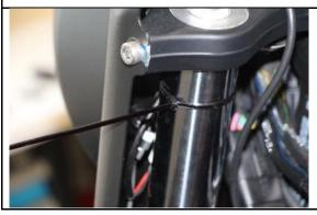
Connect the plug and attach the cables to the fork using cable ties.
