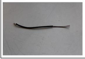
Cut the cables of the original indicators approx. 5 cm after the plug.  $\;$
