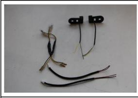
Solder all cable ends together. Use the resistors and solder connectors provided to do this.
