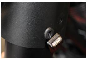
Lay the indicator cable through the rubber nozzle and behind the covering to the plug.
