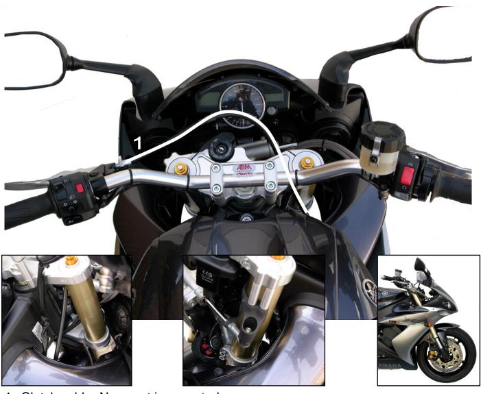
1 Clutch cable- New part is re-routed.
