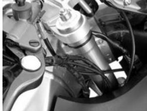
You will have to reroute the throttle cables. Resecure the wiring harness and cables in such a way that they do not limit steering lock or kink or chafe at full lock.
